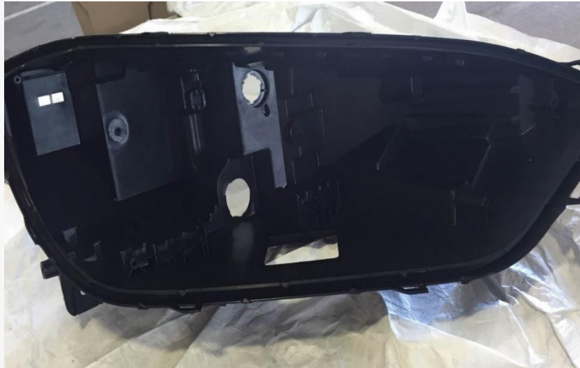
Original 40% Talc Filled Polypropylene Part – 989 grams
