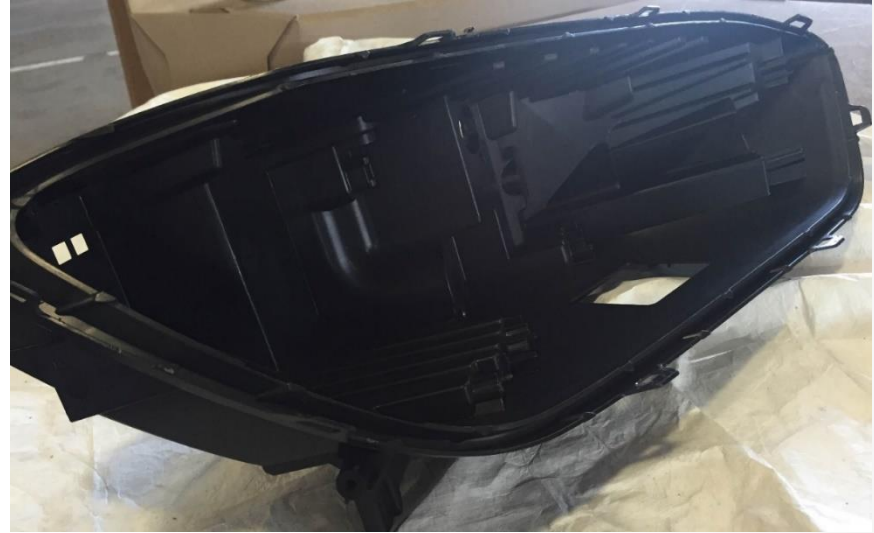
22% Bio-Carbon Filled Polypropylene Substitute – 824 grams – 17% weight saving!
